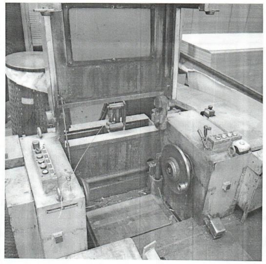
Heavy duty dynamic spooler from Herborn ideally designed for RBD drawing line. This spooler is suitable for spools of max DIN 630 mm.
